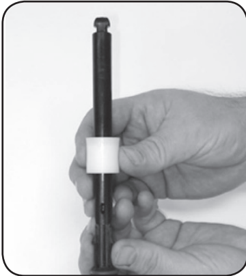
Step 4. For 2.5% & 5% Replace #44 DOSAGE PISTON flared-end up and #14 O-RING.
