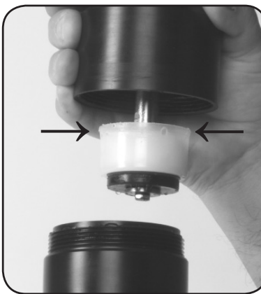
Step 7a. NOTE: #44 DOSAGE PISTON must be installed flared end up .
